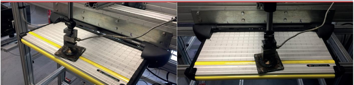
The Glide Step has undergone a rigorous series of tests to ensure safety, reliability and premium performance. This includes cycle load testing, increasing weights in both central and off-centre positions for tens of thousands of cycles.
